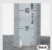
LU-1520NCS-7 (Remaining-thread length : Less than 5mm)
