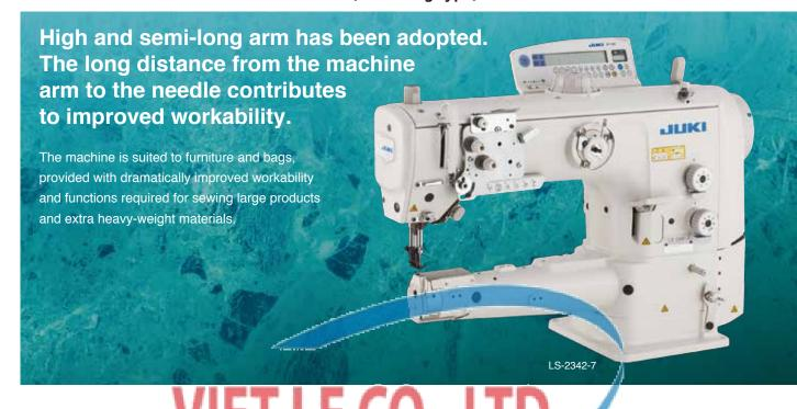
The LS-2342 offers a consistent stitching pitch and outstanding ability to sew sharp curves.
