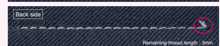
※ DDL-900BB can produce the effect of shorter-thread remaining by making condensed stitch
